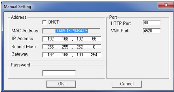
Enter the IP address, subnet mask, and default gateway. HTTP Port is used to access the camera in a web browser (the default is 80). VNP Port is used to control the video signal transfer (the default is 4520). Leave the Password box blank to keep the default password. Click OK to apply the new settings.
