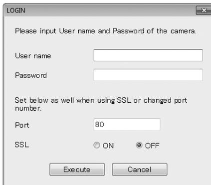
Enter the default credentials and click Execute. When you are logged in, you can assign IP information to the camera. When finished, click Execute. After the camera completes the update, the newly assigned camera information is displayed in the Search results list. **NOTE:** The factory default login for Sanyo cameras is:
