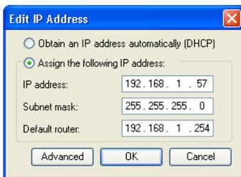
Enter the IP address, subnet mask, and default router. Click OK to apply the IP address.
