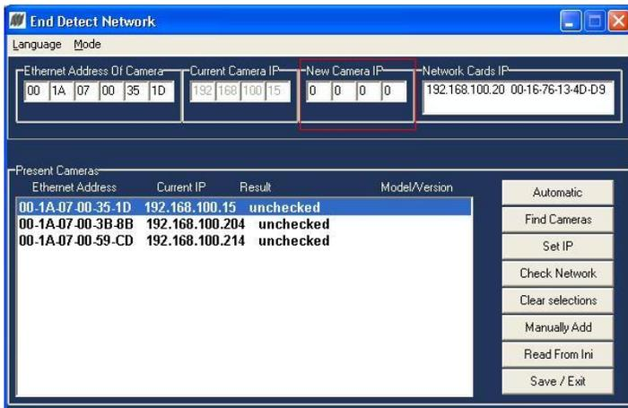
Enter the IP Address in the New Camera IP field.
