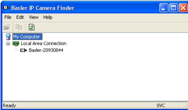
All the Basler IP cameras on the local subnet are displayed under Local Area Connection. To configure a camera, right click and select Open In Browser.
