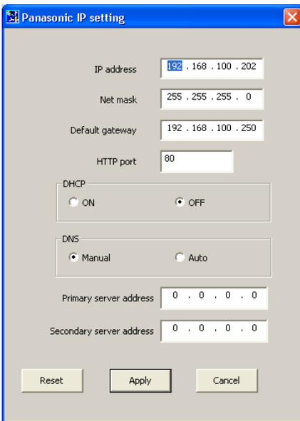
Panasonic cameras typically do not use DHCP by factory default, you must manually assign the camera an IP address. Enter an IP address that is not used by any other device on your local network, ensuring that the first three numbers match the first three numbers of your exacqVision Server's IP address. Set the net mask to 255.255.255.0, leave the HTTP port at 80, enter the camera's Administrator name and password, and click Apply.
