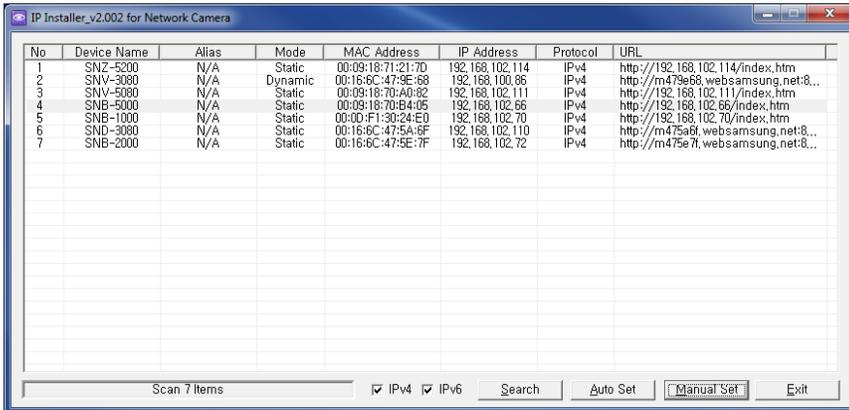
Samsung cameras on the network are listed. Click Search to update the list. To change the network settings for a camera, highlight a camera and select **Manual Set**. This opens the following window:
