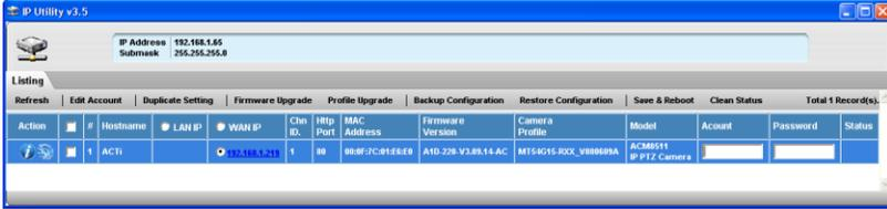
Enter the Account name and Password in the appropriate fields, and then click Configure Camera Settings (the wheel button at the far left side of the row).
