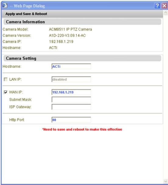
Change the WAN IP address to an IP address that is not used on your network. You cannot turn on DHCP here; that can be done only on the camera webpage. After you enter the IP address and subnet mask entered, click Apply and Save & Reboot.
