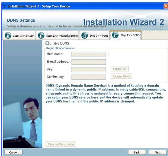
Do not select Enable DDNS unless you are planning to put this camera on the Internet. This is not recommended. Click Next to complete the configuration.
